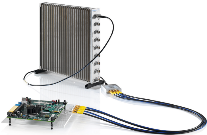
Test setup for composite MIMO TX measurement. A WLAN device with four antennas is connected to the R&S®CMW100 via a power combiner.
