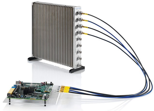
Test setup for the switched MIMO TX measurement. Each antenna in the DUT is connected to a port on one R&S®CMW100. The ports are switched in rapid succession to the test set's analyzer.
