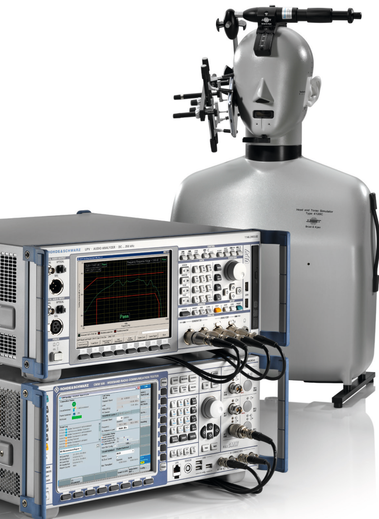
Audio analysis using the R&S®CMW500 in combination with the R&S®UPV audio analyzer.
